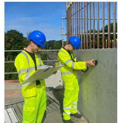
T-LEVEL STUDENTS CARRYING OUT A COVER METER SURVEY ON THE DOVER FASTRACK BRIDGE
